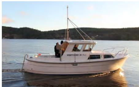
Westford 26 , Motor: 2xGS10. Battery: Lead 24V, 200 Ah Performance: 4 kn - 6 h, 5½kn - 30 min
