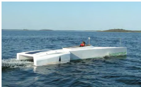
ZEB 25 , Motor: GS18. Battery: Lead 48V, 100 Ah Performance: 4 kn - 10 h, 12 kn - 45 min
