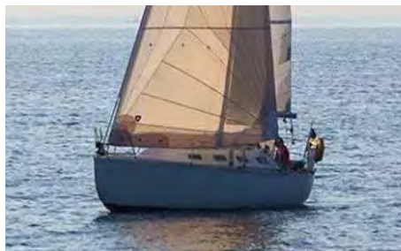
Grinde , Motor: GS10. Battery: Litium 24V, 100 Ah Performance: 4 kn - 3½ h, 5½ kn - 40 min
