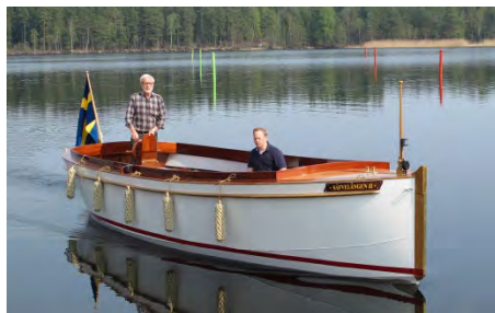
Säfvelången II , Motor: GS18. Battery: Lead 48V, 200 Ah Performance: 4 kn - 11 h, 6 kn - 2 h
