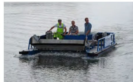
RenStröm , Motor: 2xGS18. Battery: Litium 48V, 360 Ah Performance: 4 kn - 16 h, 5½ kn - 2 h
