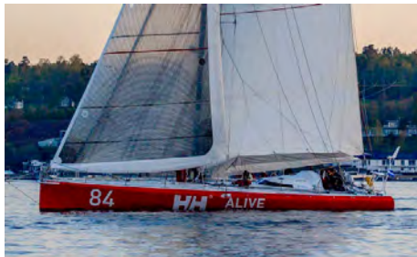
Open 60 , Motor: E35P. Battery: Litium 48V, 160 Ah Performance: 4 kn - 3½ h, 5 kn - 1 h
