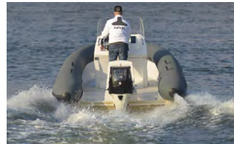
Hava 700 , Motor: BO200P. Battery: Litium 350V, 160 Ah Performance: 20 kn - 2 h, 35 kn - 30 min
