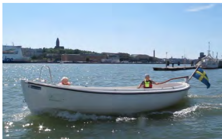
Vikensnipa , Motor: GS10. Battery: Litium 24V, 200 Ah Performance: 4 kn - 11 h, 6 kn - 1½ h
