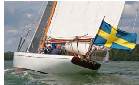
RIO , Motor: 2xGS18. Battery: Lead 48V, 400 Ah Performance: 4 ½ kn - 13 h, 6 1/2 kn - 1 h
