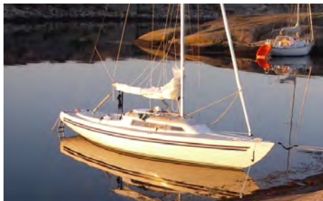
H-Båt , Motor: GS10. Battery: Lead 24V, 100 Ah Performance: 4 kn - 3½ h, 6 kn - 20 min
