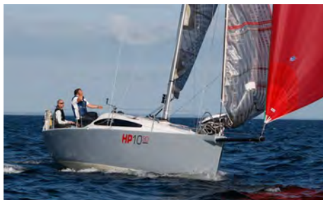
HPI030 , Motor: GS10. Battery: Lead 24V, 200 Ah Performance: 4 kn - 7 h, 6 kn - 40 min
