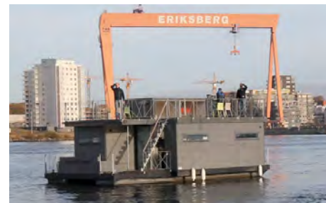
Ocean Living Motor: 2xGS18. Battery: Lead 48V, 800 Ah Performance: 3 kn - 7 h, 4 kn - 1½ h
